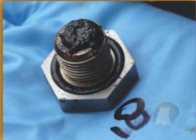
Biofilm present on a carbon steel biostud located in a produced water system
