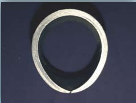
Figure 1: Side and cross sectional views of a failure, showing multiple bulges and a rupture at a bulge apex
